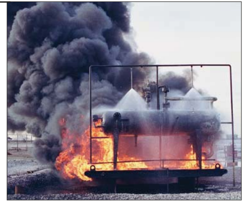
N6 nozzles protect a propane storage tank from fire and explosion.
