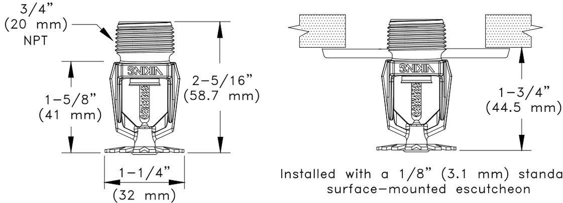
Figure 2: Sprinkler Dimensions
