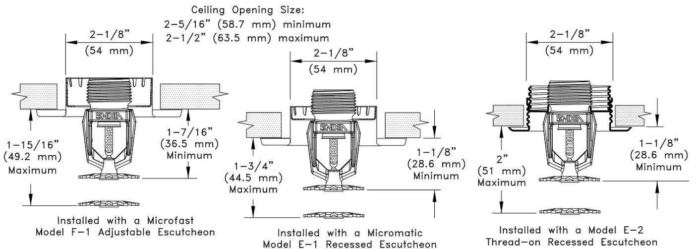
Figure 3: Pendant Sprinkler VK536 Dimensions with the Model F-1, Model E-1 and E-2 Recessed Escutcheons
