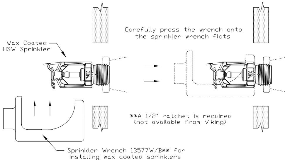
**Figure 3: Wrench 13577W/B for Wax Coated Sprinklers**
