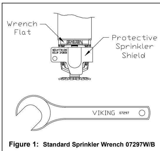
Figure 1: Standard Sprinkler Wrench 07297W/B
