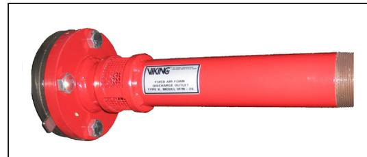
The Foam Makers incorporate an orifice, air inlet and mixing barrel. The body and orifice are corrosion resistant brass. The air inlet screen is corrosion resistant stainless steel.
